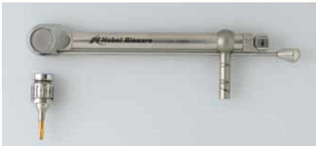
Fig. 6 Ratchet with spring rod that accommodates different bits and offers a reversing option at the end of the handle (Nobel Biocare, Cologne).
